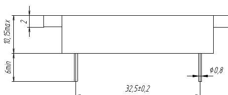
Dimensions in mm. This dimensional layout refers to single-output version with flanges. Dual- and triple-output models are also available.
