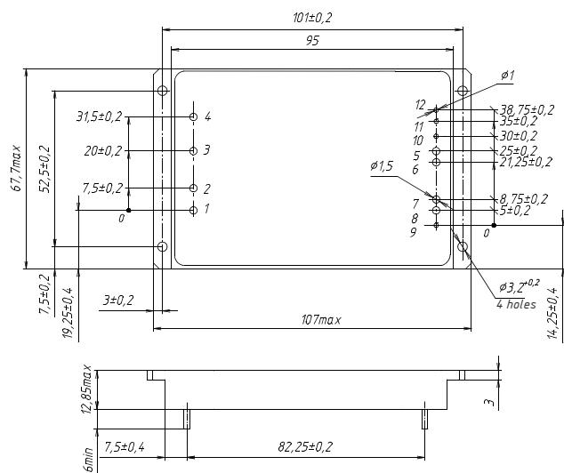
Dimensions in mm. This dimensional layout refers to units of 80 W and 160 W. Dimensional layout of 120 W model can be found in technical documentation on the manufacturer's website.
