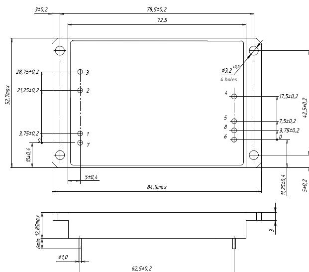
Dimensions in mm. This dimensional layout refers to single-output version. Dual-output model is also available. Detailed information can be found in technical documentation on the manufacturer's website.
