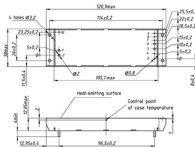
Module with vertical pin out, case with flanges "U" type. Dimensions in mm. Case version with "D" type flanges is also available. Detailed information can be found in technical documentation on the manufacturer's website.
