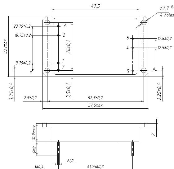
Dimensions in mm. This dimensional layout refers to single-output version with flanges. Dual-output models are also available. Detailed information can be found in technical documentation on the manufacturer's website.
