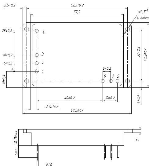
Dimensions in mm. This dimensional layout refers to single-output version with flanges. Dual-output models are also available. Detailed information can be found in technical documentation on the manufacturer's website.
