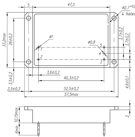
Dimensions in mm. MDF100 model layout. Description of pins can be found in manufacturer's engineering documentation.
